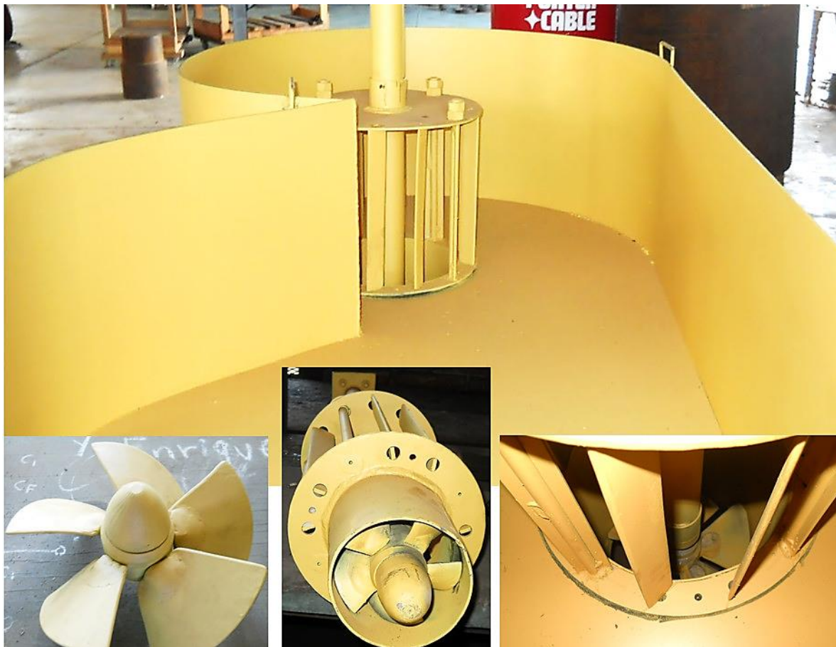
[6.7] Axial turbine fabricated in León, Nicaragua (author's photos)
