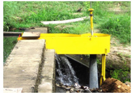
[6.8] Installation of an axial “Simplex” in León, Nicaragua 2012 (author’s photos)
