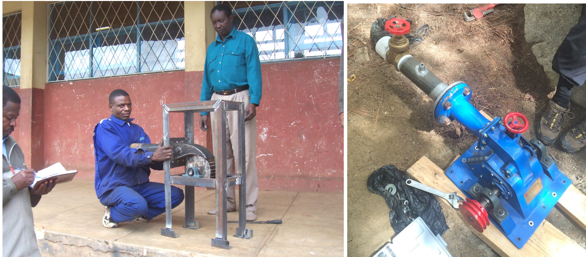
[6.11] Michell Banki Turbine fabrication in Mozambique (Gnecco, 2012)
