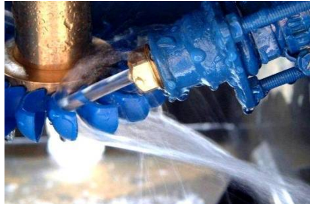
[6.24] Water Flow through a Turgo Turbine Runner (ESHA, 1998: 158)
