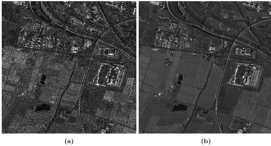
Figure 2.5: SLC image speckle example. (a) Original SLC amplitude and (b) time averaged amplitude from an SLC stack.
