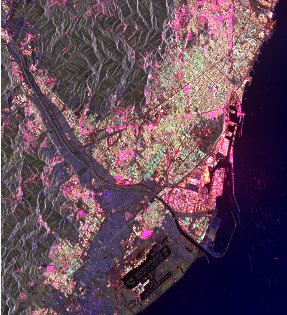
Figure 3.6: Pauli RGB representation of Barcelona. Composite of channels P1 (Blue), P2 (Red) and P3 (Green).
