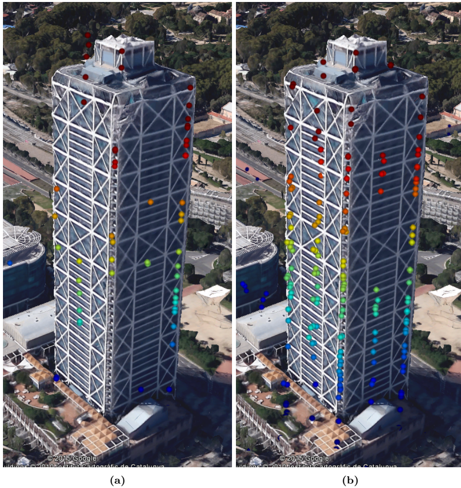
Figure 6.4: Topographic error in Hotel Arts. Results for the HH data-set 6.4a and for the ESM-MB data-set. 6.4b.
