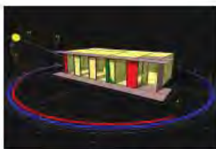
Detailed Shading analysis of an apartment with Ecotect. Winter time. January 15th Solar penetration is allowed
