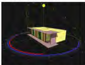
Detailed Shading analysis of an apartment with Ecotect. Summer time. August 15th Solar direct radiation is blocked by the overhang
