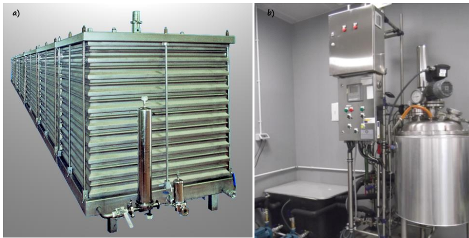
Figure 4. Pilot plant equipment commonly used in producing BCAs in a) solid (Bayer CropScience, Germany) and b) liquid state.
