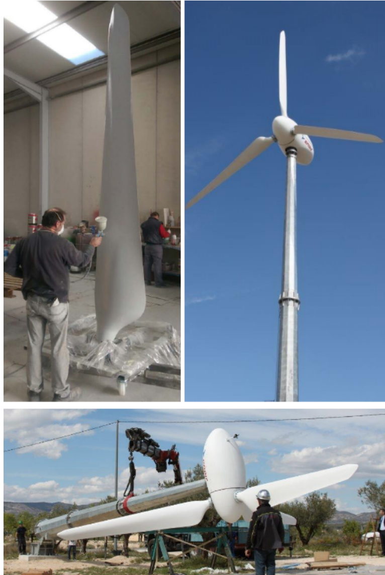
Figure A.8: Images of the 10 kW machine. Left: ultimate blade treatment. Bottom: erecting process. Right: final layout of the turbine ready for testing and operation.
