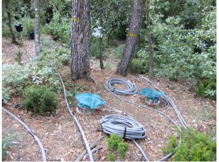
Figure 4.1. One pair of soil chambers, the right one is to measure heterotrophic respiration, with PVC tube as trench, while the left one is to measure the total soil respiration. (Photo: C.-T. Chang)
