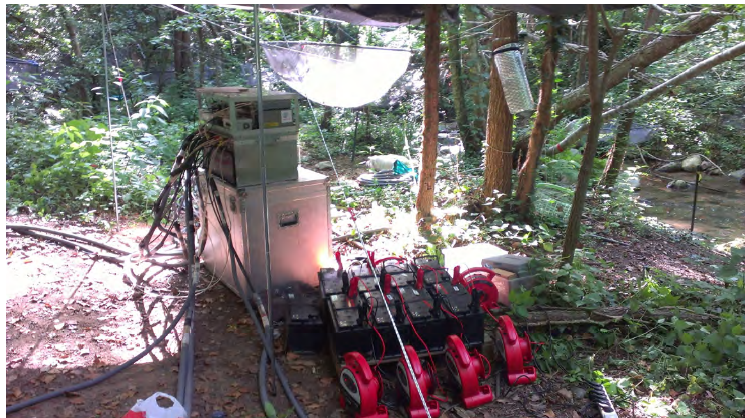
Top: automatic changeover open system and batteries. System power was supplied by six batteries. Photo:C.-T. Chang
