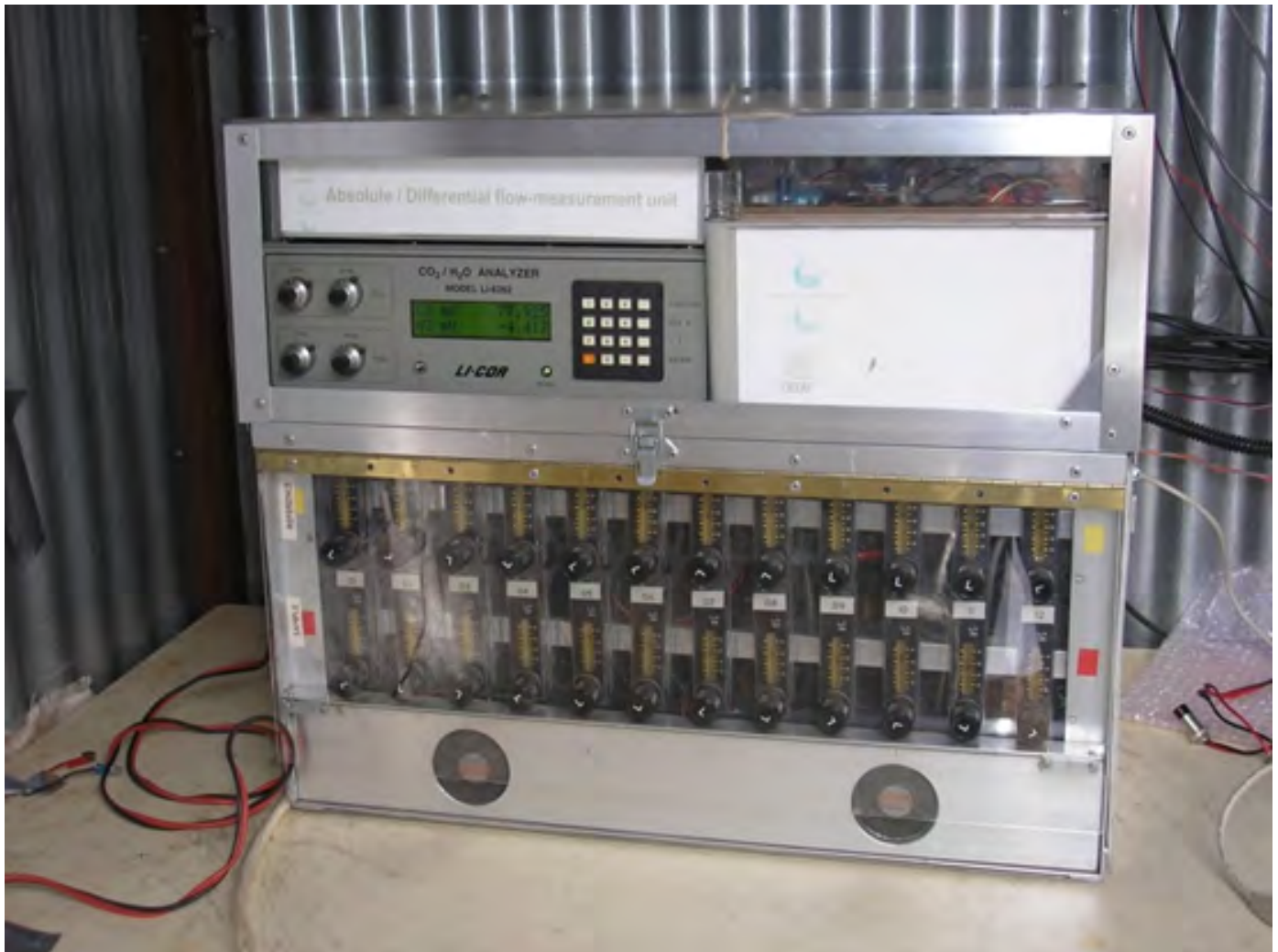
Figure 3.3. The automatic changeover open system. The upper left is IRGA, upper right is the cataloguer. The lower part is the rotameters, pumps and flowmeters. (Photo: S. Sabaté)
