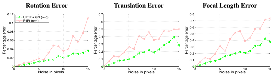
Figure 3.10: Comparison of the UPnP using 6 correspondences vs. the minimal approach proposed in [7], which estimates pose and focal length from four 3D-to-2D correspondences.
