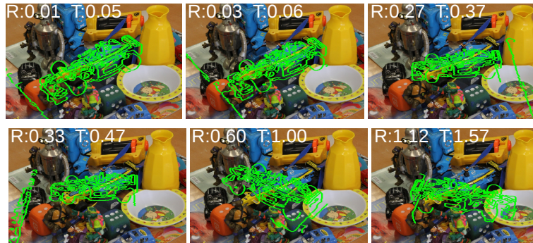
Figure 5.8: We show examples of increasing amounts of error to ease the understanding of the result charts. R is for rotation error and T is for translation error. The image shows the error between a test image and one of the training images. Edges from the corresponding training image are superposed on the test image to show the variation of pose. For clarity, we have used the same test image to make comparison of the error magnitudes easy. This figure is purely informative and the errors shown are not the actual errors yielded by our approach or any of the baselines.
