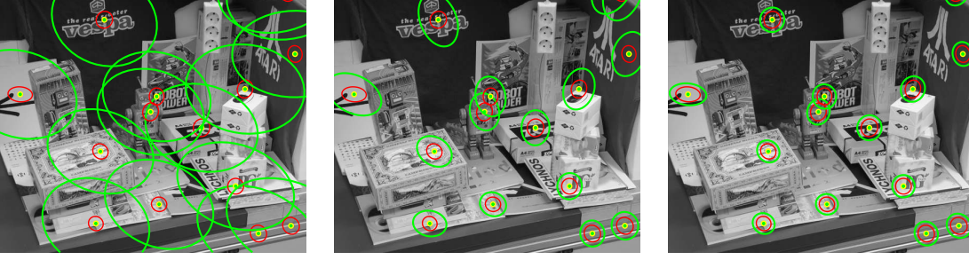
Figure 4.3: Limiting the number of potential candidates. Left: Search region obtained after projecting the three terms of Eq. 4.2 independently. Center and Right: Refinement of the search space, after establishing correspondences.
