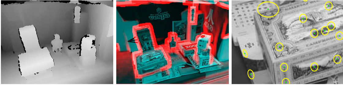
Figure 4.2: Uncertain 3D model. Left: 3D model acquired with a Kinect camera. Regions in which the 3D data is most uncertain are depth discontinuities. Center: We detect the uncertain regions –shown in red– computing depth covariances within local neighborhoods. Right: A 3D covariance is assigned to each 3D model point and propagated to the image plane. This is used to limit the area where to search for potential match candidates.
