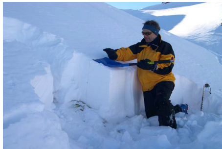
(a) Compression test
