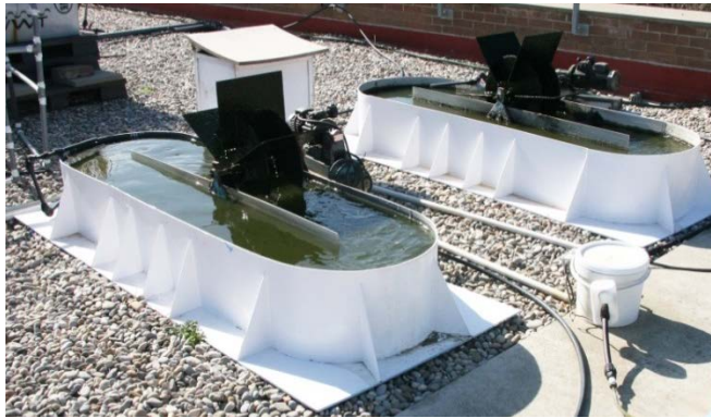
Figure 1.3 Experimental high rate algal ponds on the roof of the GEMMA group building at UPC in Barcelona (Spain).
