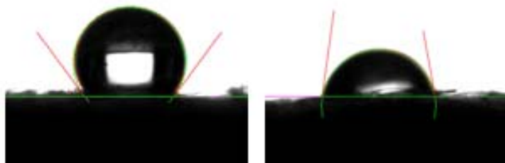
Figure II.22. Contact angle measurement.
