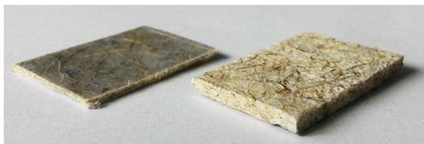
Composite material: before foaming (left) and after foaming (right).
