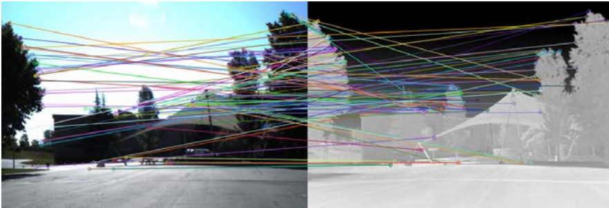
Figure 1.1: The figure shows the result of performing feature matching between a visible and an LWIR image using SIFT. Visible image at the left and LWIR at the right.
