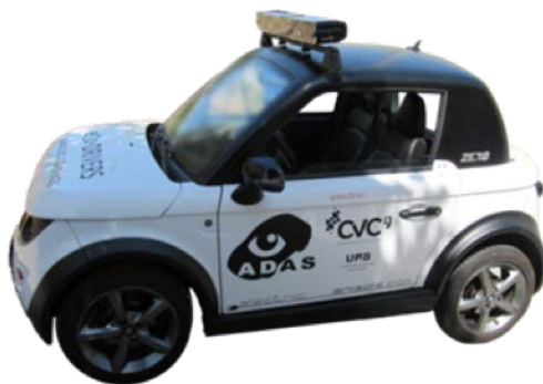
Figure 3.8: Electric car used to capture the VIS-LWIR multi-spectral odometry dataset. Cameras are mounted on the roof.
