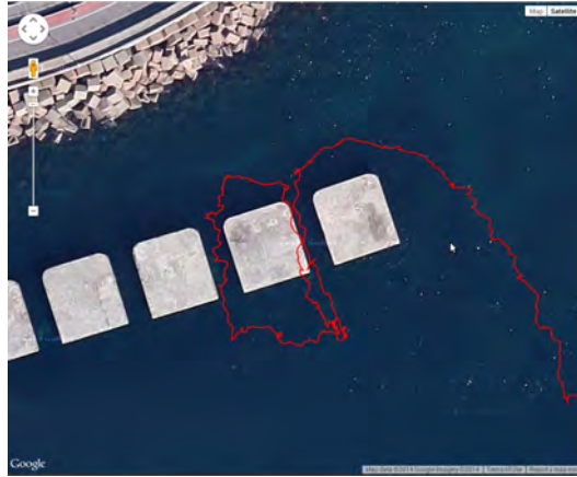
Figure 57: Sparus II AUV was teleoperated at surface in the breakwater structure scenario. Although the Sparus II did not collide during the teleoperated mission, GPS data (in red) shows a vehicle trajectory under collision with and even over the concrete blocks. Satellite view. Image credit: Map data ©2017 Google.
