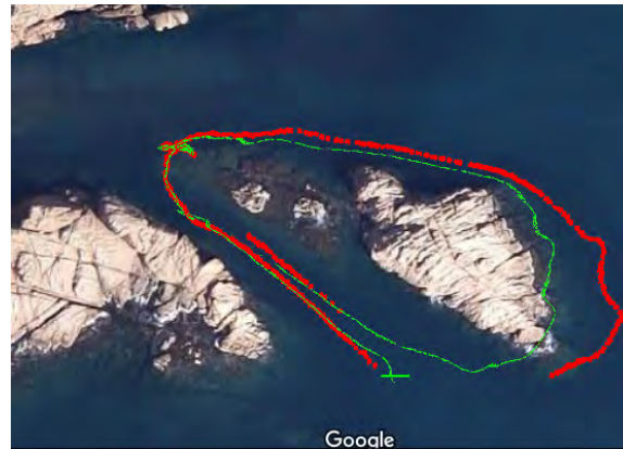
Figure 65: Vehicle trajectory (green) calculated by its dead-reckoning system and the camera trajectory (red) estimated by the image-based reconstruction. Both trajectories are shown overlapped with a satellite image of the test scenario (Map data ©2017 Google).
