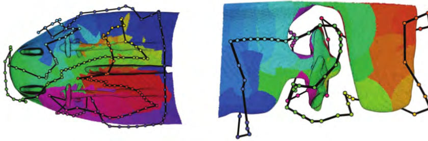
Figure 17: Coverage path planning (CPP) algorithms are normally used to plan routes to inspect different kind of structures. In most of these applications the planner has preliminary information. This may include a 2D/3D map of the area or structure to be inspected.
