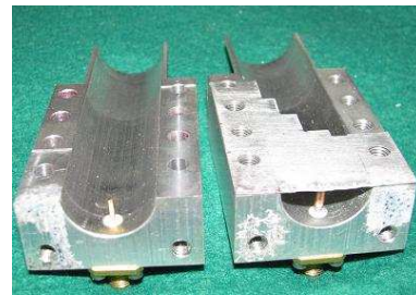
(B) Real horn with Septum polarizer disassembled.
