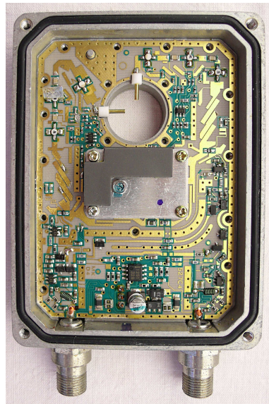
(A) LNB with two ortho- gonal monopo- les.
