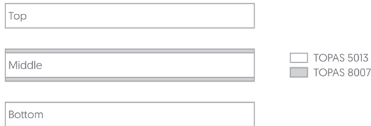
Figure 3.11: Schematic cross-section view of the layers of the device for E. coli detection. The middle layer is laminated with TOPAS 8007 prior to microstructuring in order to facilitate the bonding process. Not to scale.
