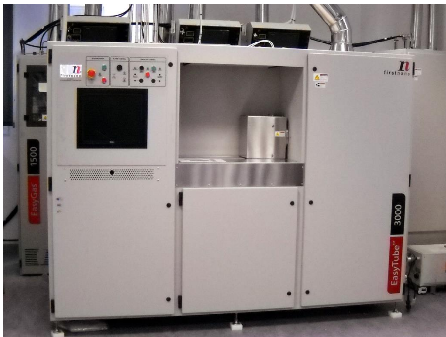
Fig. 9. CVD reactor EasyTube 3000 from FirstNano at IREC facilities, employed for nanostructure growth in this work Table 1 summarizes the properties of the gases fed to the in the CVD reactor during the nanostructure growth processes carried in this work.
