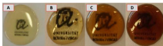
Figure 8. Photographs of the thermosets obtained from different ECC/thiol formulations catalyzed by 2 phr of DMAP: A) 6SH-SQ; B) PETMP; C) 3SH-ISO and D) 3SH-EU
