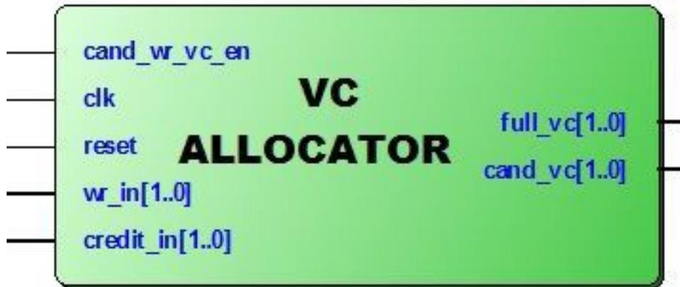
FIGURE 6.8: Symbol of Virtual Channel Allocator Module
