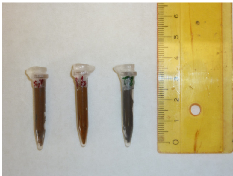
Figure 4.3: Three 400 \mu\text{l} sample vials (sludge at 6.9m, sludge at 8.15m and tailings at 8.5m depth) for bulk XANES and XRF measurements.
