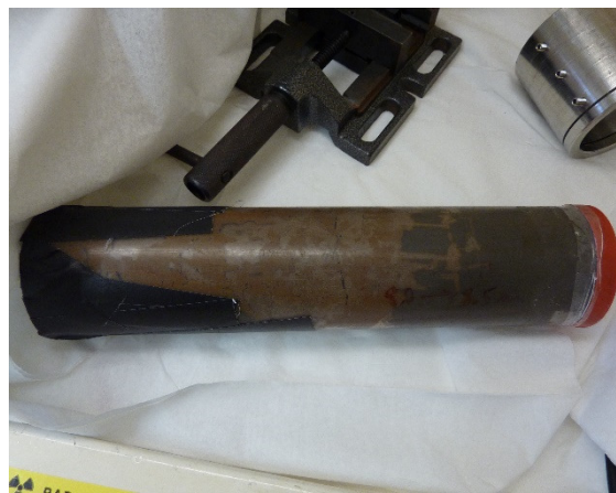
d) Interface between sludge and tailings at 8.3 m depth
