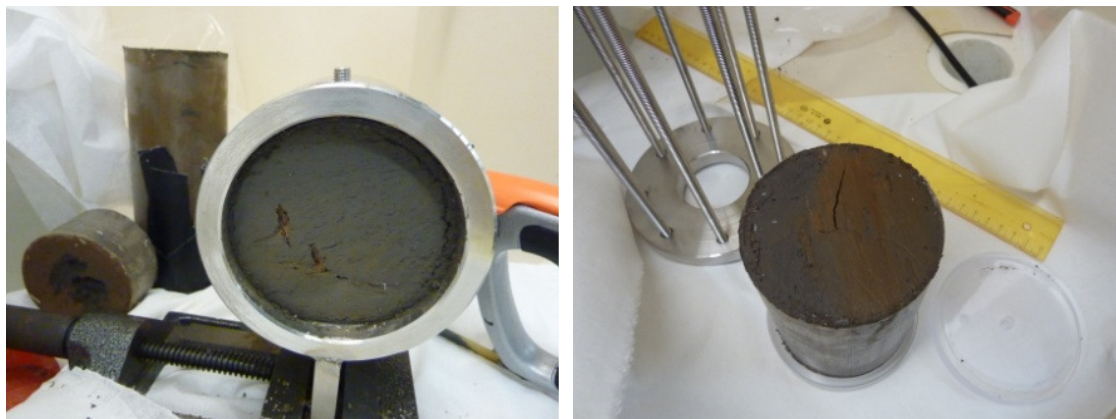
Figure 8.9: Base (on the left) and top (on the right) of the undisturbed column of tailings, Core B, showing irregularities and a fracture in the material.
