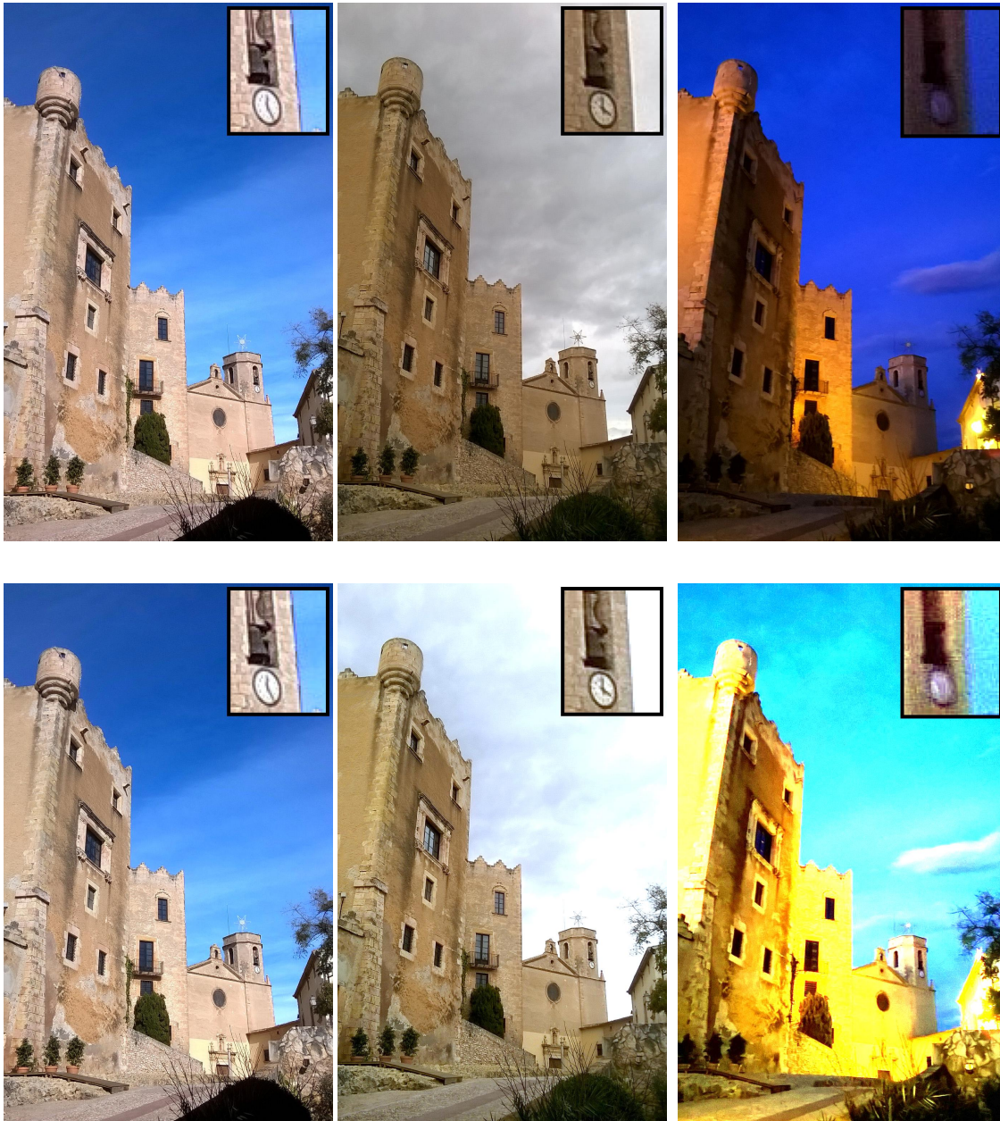
Fig. 16 The normalisation problem. The top row shows three images of Altafulla castle taken in different light conditions. All three have been normalised to stretch the dynamic range to the maximum [0,255] and a region of interest is shown with the detail of the clock and bell in the church steeple (rightmost building).
