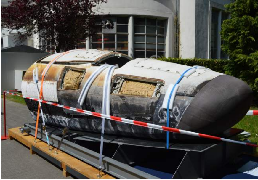
Figure 6.10.: Photograph of IXV after re-entry, taken at the VKI on June 2015.
