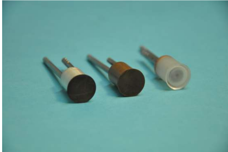
Figure 3.9.: Calorimeters for Mini-Max methodology application: left - Ag, middle - Cu, right - SiO 2 -Quartz.
