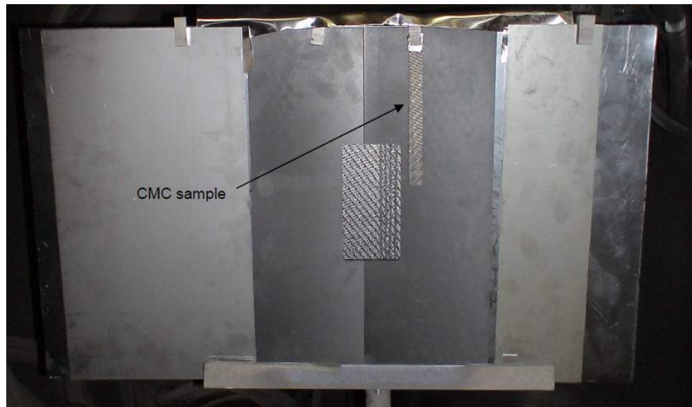
Figure 6.5.: Graphite mask on shingle 5 before coating with a CMC sample attached for qualification.
