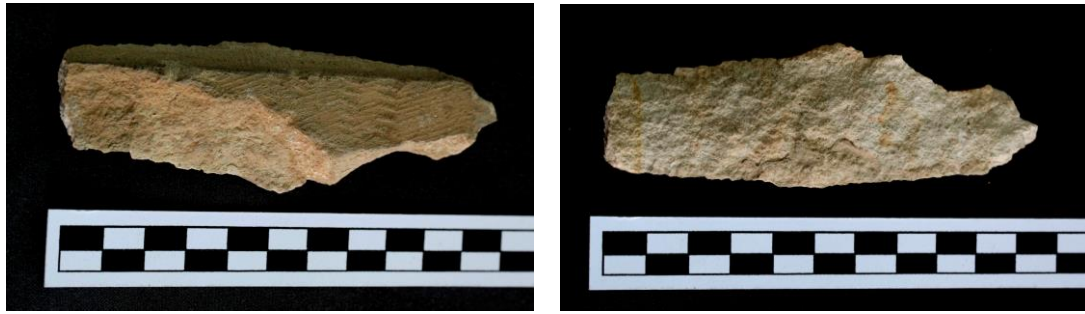
Figure 2. Example of an original stone fragment used in the evaluation of treatments consolidation. The treatments were applied on the obverse surface (with artificial patina) and the reverse surface (natural stone).
