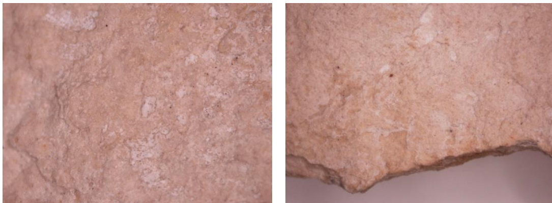
Figure 6. Stereomicroscopy image of the reverse surface treated with alcoholic suspension of hydroxide nanolime (A), and the reverse surface treated with aqueous suspension of barium hydroxide (B).
