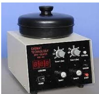
*Figura 3. 8 spin coater KW-4A chemat technology.*
