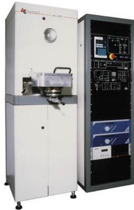
Figura 3. 1 DC magnetron sputtering Ac450 Alliance Concepts[194].
