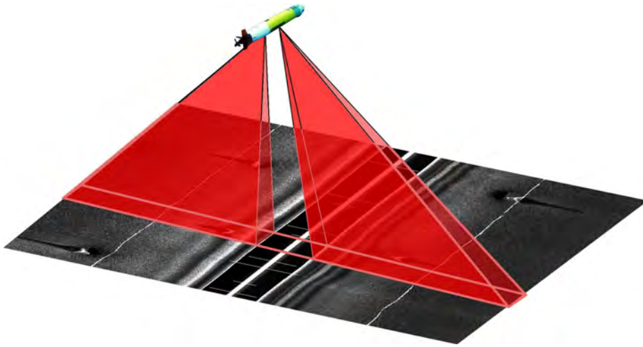
Figure 4.17: The side-scan sonar working principle.
