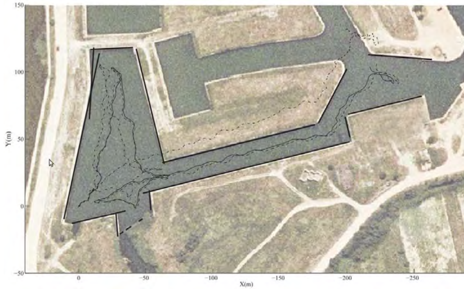
Figure 4.2: Example of a line feature based SLAM approach [Ribas 2008b]. The image shows the resulting map together with the dead-reckoning (dash-dotted line), GPS (dashed line) and SLAM (solid line) trajectories represented in a satellite image of the scenario.
