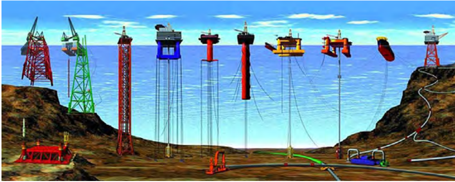
Figure 1.1: Types of offshore oil and gas structures: 1, 2) conventional fixed platforms; 3) compliant tower; 4, 5) vertically moored tension leg and mini-tension leg platform; 6) Spar ; 7,8) Semi-submersibles ; 9) Floating production, storage, and offloading facility; 10) sub-sea completion and tie-back to host facility [NOAA 2008].
