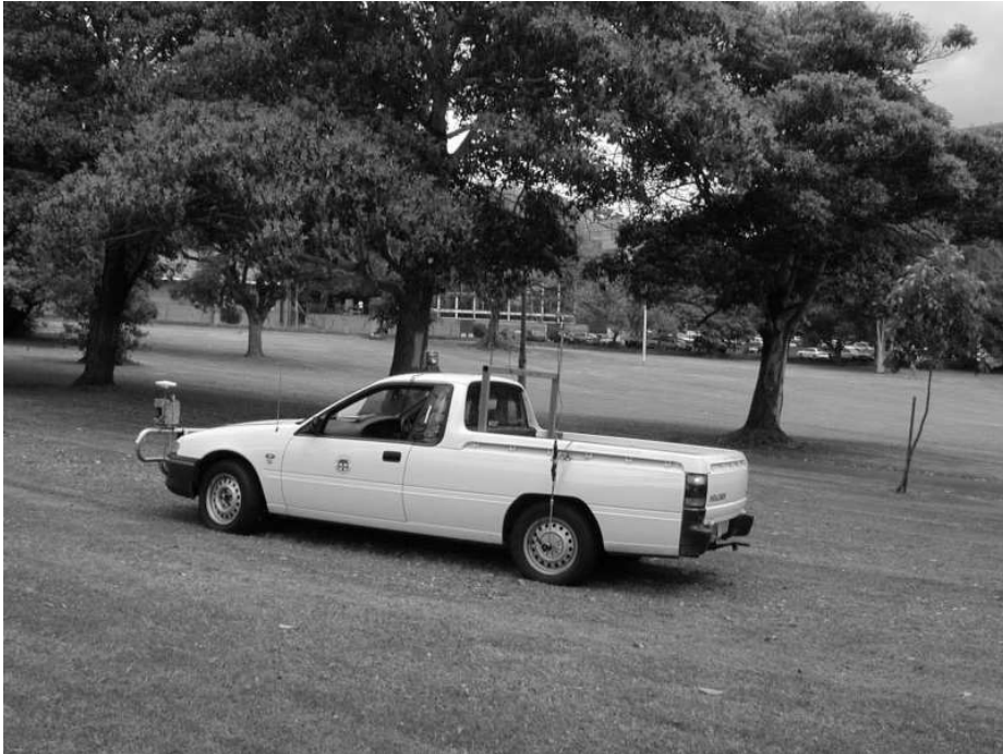
Figure 3.8: Utility vehicle used to gather the Victoria Park dataset. The vehicle is carrying the scanning laser sensor (vehicle left front) and the optical speedometer (left back wheel) (source: [Guivant 2002b]).
