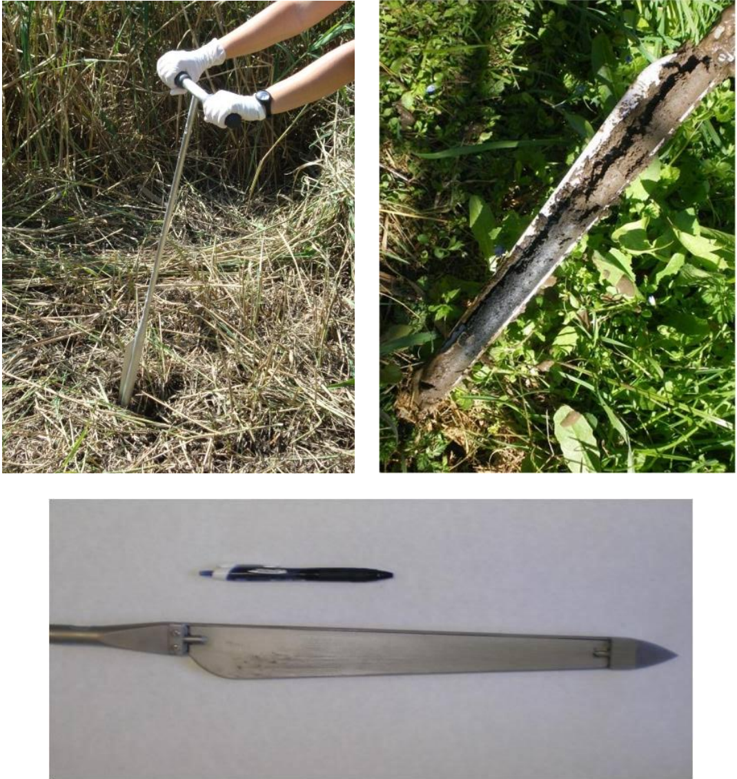
Figure 4.3 Details of the Eijkelkamp soil coring kit and of one collected sample.
