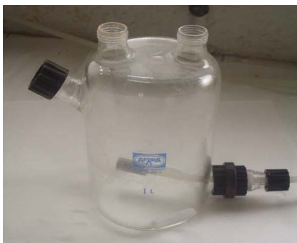
Figure III.2 LFS respirometric vessel
