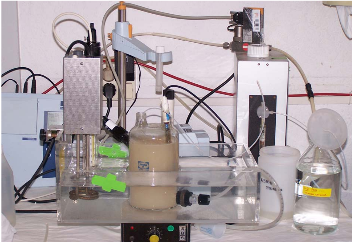
Figure III.3 Overview of the whole LFS respirometer equipment
