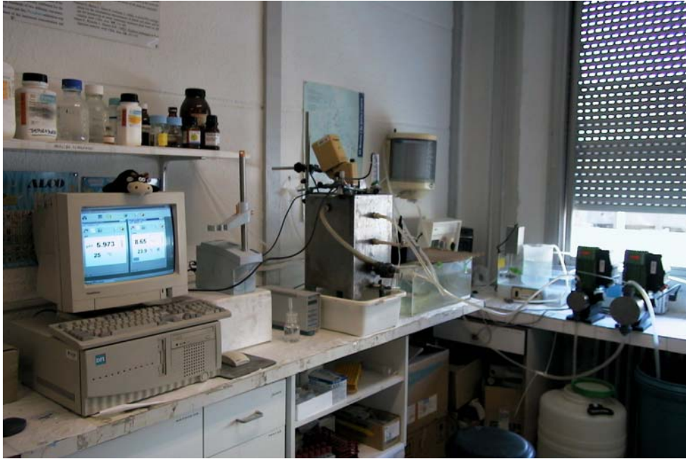
Figure III.12 Overview of the aerobic-SBR equipment.
