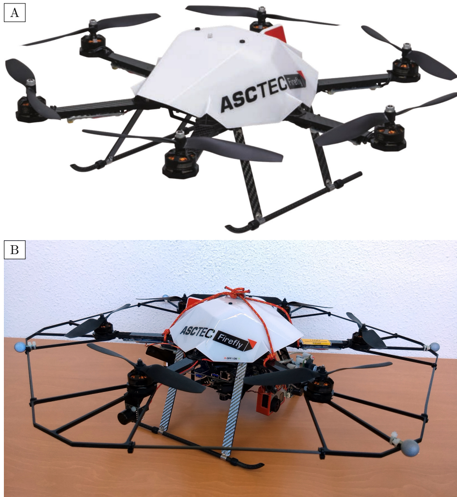
Figure 3.18: The AscTec Firefly platform: (A) the aerial platform as delivered by the manufacturer, and (B) the platform equipped with the SS1, an on-board computer and an additional camera for video recording.
