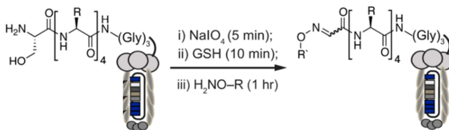
Figure 4. Chemical modification of the phage-displayed peptide library through oxime ligation to an N -terminal glyoxal generated by NaIO 4 oxidation of N -terminal serine. R = aminoacid side chain; R' = manose, biotin, sulfonamide. 30
