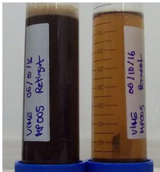
Figure 3.49: Retained and permeate samples for membrane 6 test
