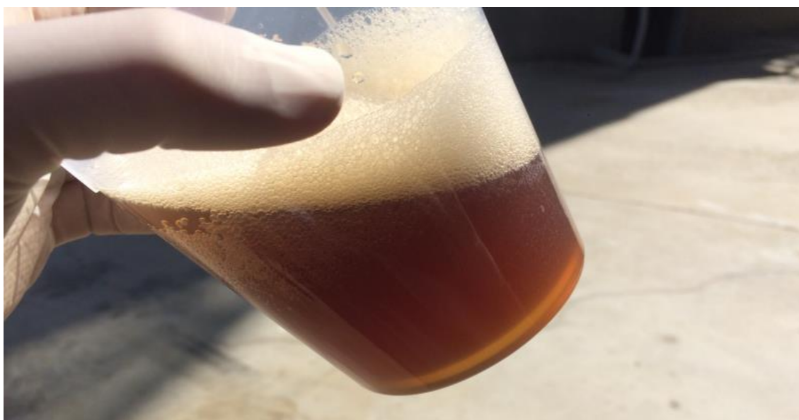
Figure 2.7: Liquid phase aspect obtained with flocculant FLOPAM TE 4650 SH (test 3)
