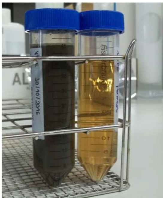
Figure 3.79: Retained and permeate samples for membrane 12 test
