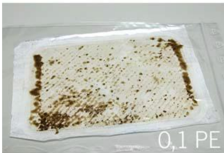
Figure 3.78: Photograph of membrane 12 after test
