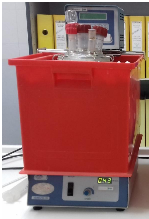
Figure 9: Assembly for the thermal hydrolysis tests
