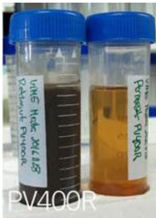
Figure 3.64: Retained and permeate samples for membrane 9 test
