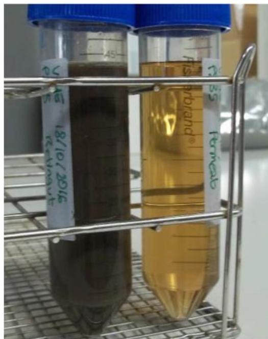
Figure 3.24: Retained and permeate samples from membrane 1 test
