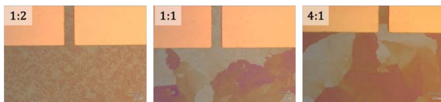
Fig. 7.3: Optical images of three different devices fabricated using different C8-BTBT:PS ratios (1:2, 1:1 and 4:1).
