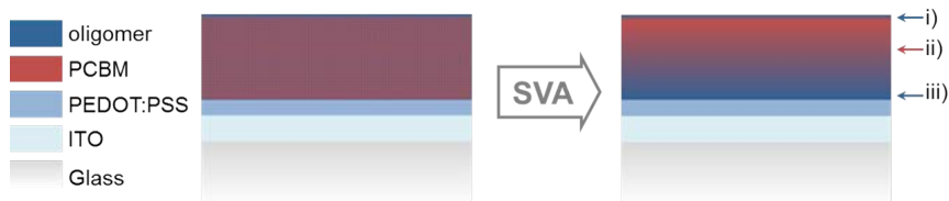
Fig. 6.13: Scheme of the vertical configuration of the oligomer 2:PC 61 BM or PC 71 BM solar cells. For the solvent-vapor annealed sample three regions are marked: i) oligomer-enriched surface, ii) sub-surface region with decreased concentration of oligomer, iii) a slightly oligomer-enriched region up to the bottom interface.
