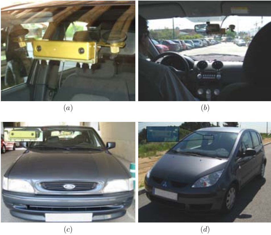
Figure A.2: Acquisition system. (a) Camera. (b) View from inside of the vehicle. (c, d) The two acquisition vehicles used.
