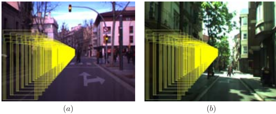
Figure 3.9: Results of the Flat World Assumption algorithm (in order to enhance the visualization just the row of X_W = -3 m is shown). (a) The grid coincides with the real road plane, so all pedestrians are correctly framed. (b) The estimated road plane does not match with the real one, so far pedestrians are not selected as candidates.
