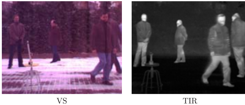
Figure 2.1: Appearance of VS and TIR for the same scene. As can be seen, the former provides color and textures while the latter highlights the higher temperature of the human body (Photo by ADAS Group, Universitat Autònoma de Barcelona and Universidad de Alcalá de Henares).
