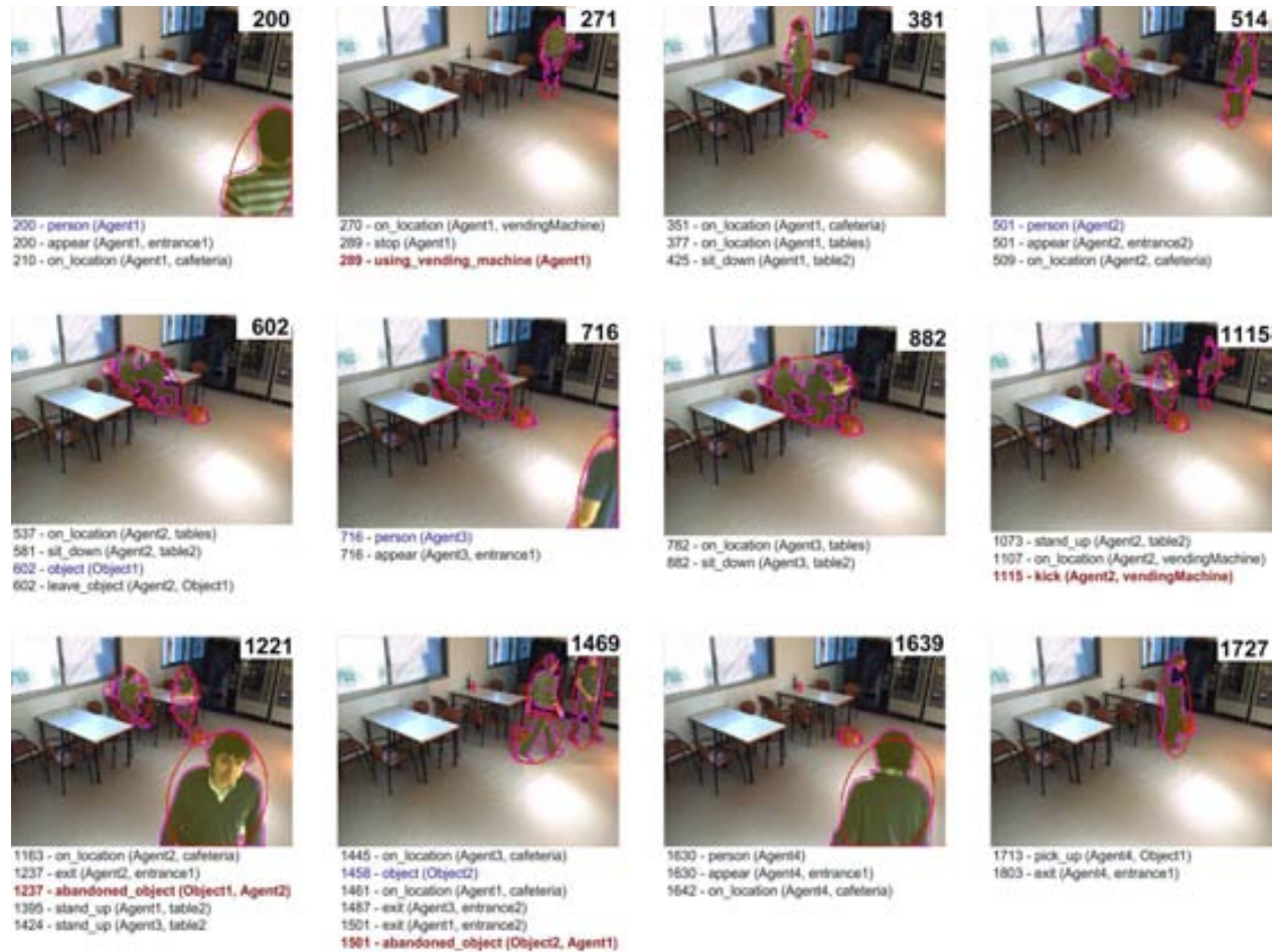
Figure 4.13: Set of semantic annotations produced for the indoor scene, which have been automatically generated for the fragment of recording comprised between frames 150 and 1839.
