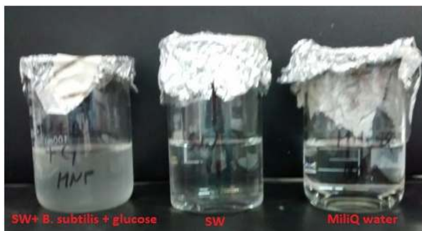
Figure 8.11. Solutions under study after 24 hours of incubation, from the left to the right: seawater with glucose and Bacillus subtilis , seawater, MiliQ water.
