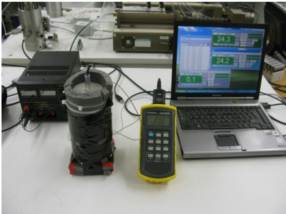
Figure 4-7 Thermal conductivity test experimental set-up. From left to right: power supply, the sample being tested with the needle probe placed in its centre, digital thermometer (yellow frame), and computer. (Pintado et al., 2013)
