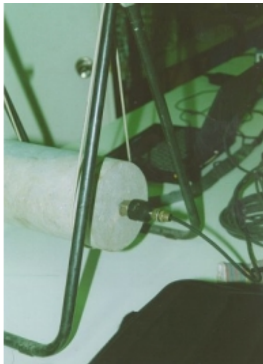
Figure 6.6.3. Stone cylinder (15x30 cm) suspended to identify dynamic strain modulus (ASTM C-215)
