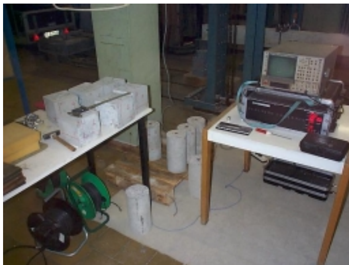
Figure 6.3.14. ASTM C215 test to obtain dynamic strain modulus. Acquisition system.
