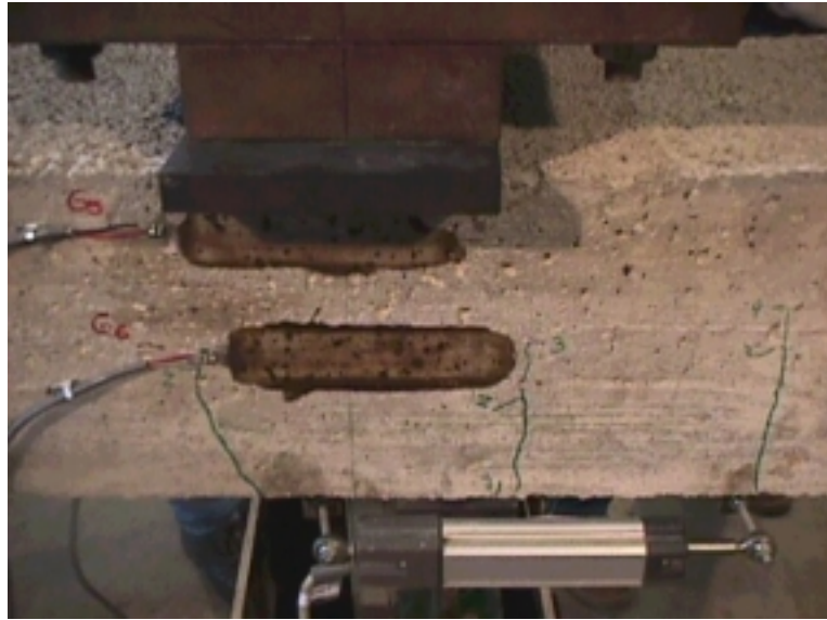
Figure 6.2.10. Attached strain gauges and displacement transducers.
