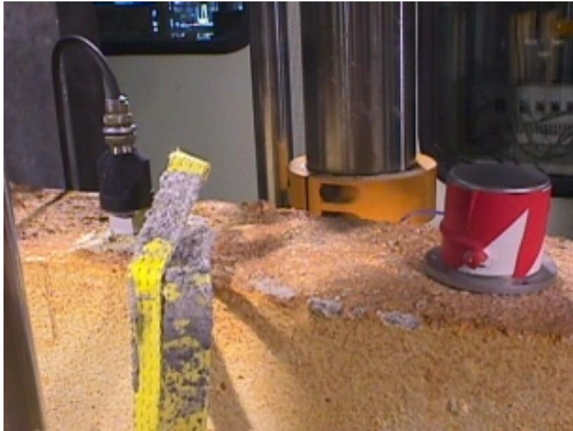
Figure 6.4.10. Attached accelerometers on beam's dynamic testing.
