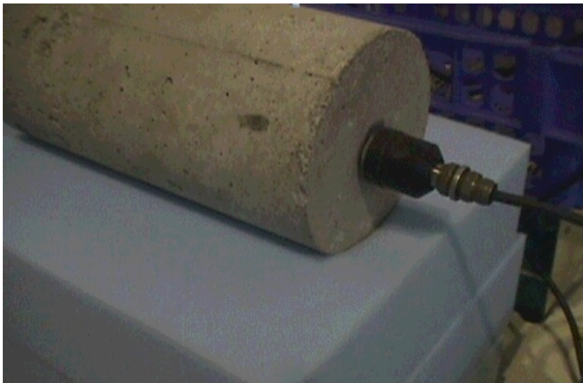
Figure 6.2.6. Identification of the longitudinal frequency in cylinders to calculate dynamic elasticity modulus.
