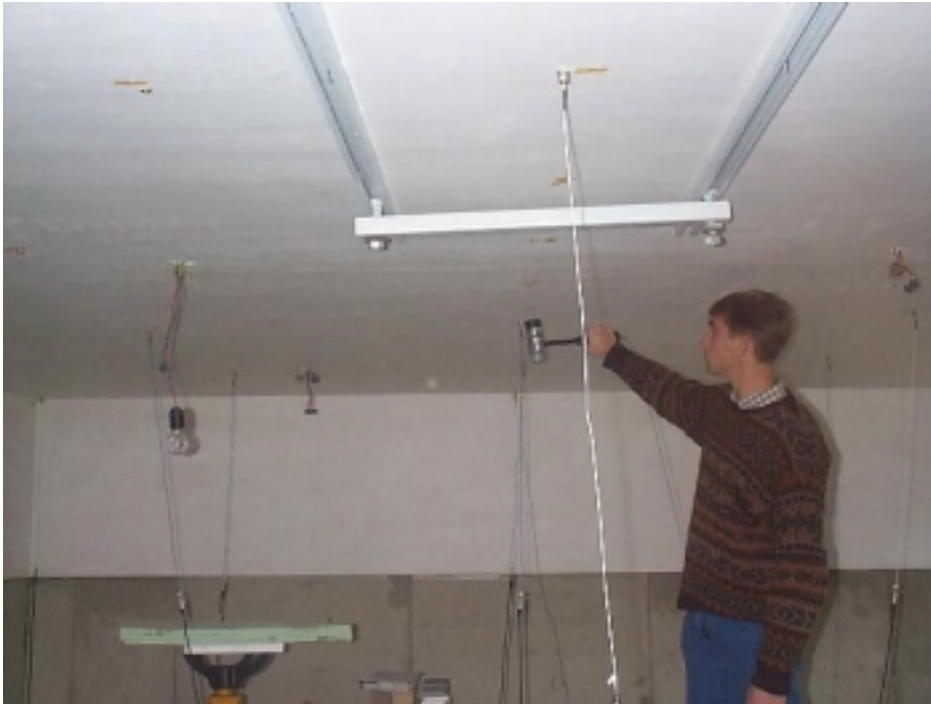
Figure 7.5 Excitation of the slab by impact-hammer.
