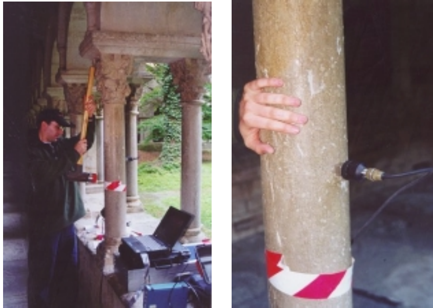
Figure 7.28. Acquisition system (left) and accelerometer attached on a column (right)
