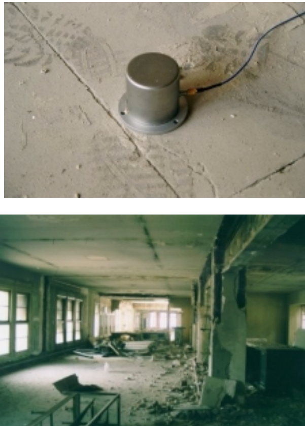
Figure 7.17. Accelerometer attached to the slab(above) and view of the tested slabs(below)
