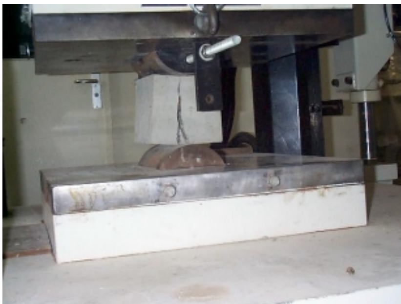
Figure 6.3.9. Brazilian test on cubes to obtain tensile strength of concrete.
