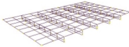
Figure 7.12. FEM of the evaluated hall slab
