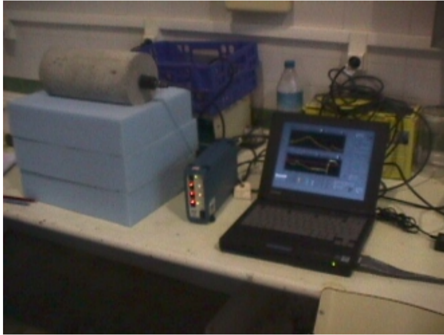
Figure 6.4.15. Dynamic-modulus testing of cylinders (C215 test of ASTM).
