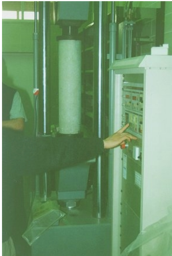
Figure 6.6.1. Loading process of the stone column.
