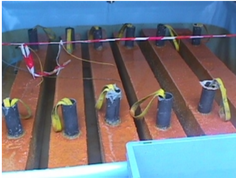
Figure 6.4.4. Beams subjected to attack ( \text{SO}_4 ) inside the pool.
