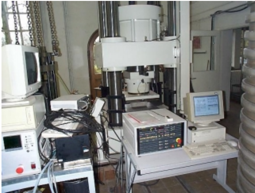
Figure 6.3.8. Brazilian test, Acquisition and loading systems.
