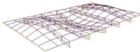
Figure 7.13. First three modal shapes of hall slab model.
