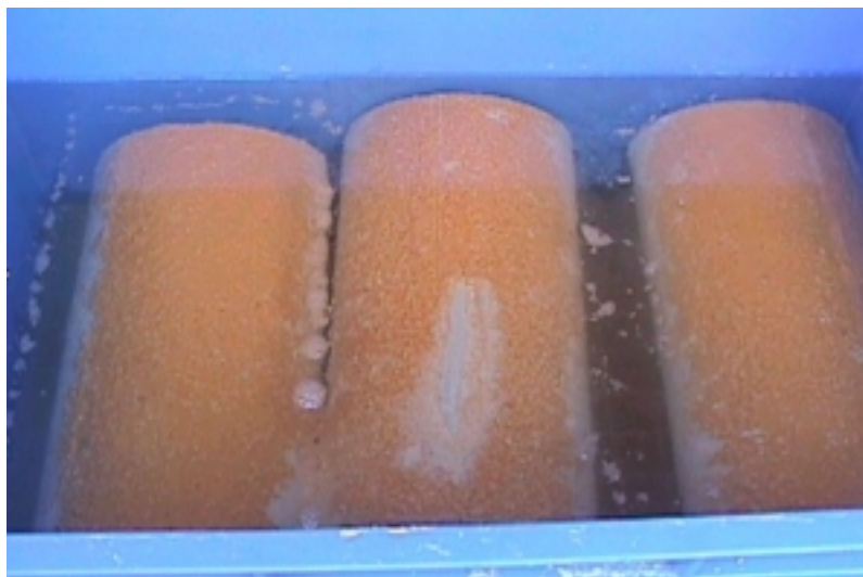
Figure 6.4.5. Attack containers for cylinders ( \text{SO}_4 ).
