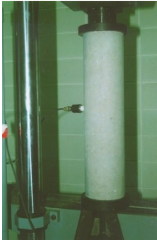
Figure 6.6.2. Quartz accelerometer attached to the tested stone column.
