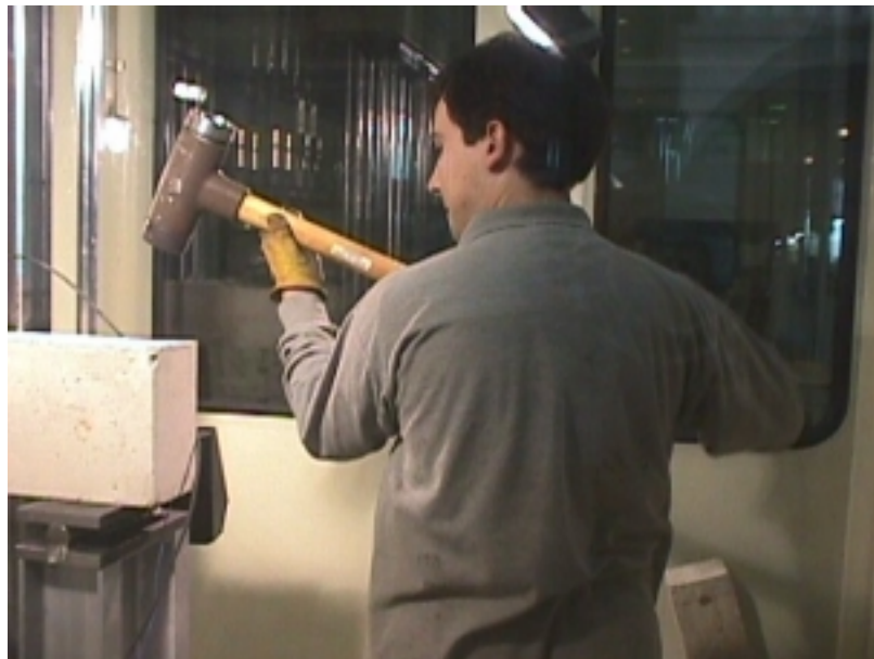
Figure 6.4.11. Excitation of the beam by hammer impact.
