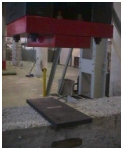
Figure 6.2.9. Neoprene element used to regularize the load.
