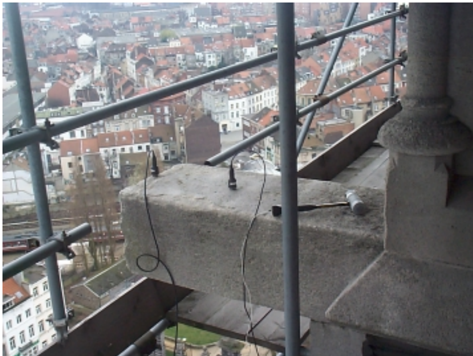
Figure 7.48. Instrumentation of one stone with 2 sensors.
