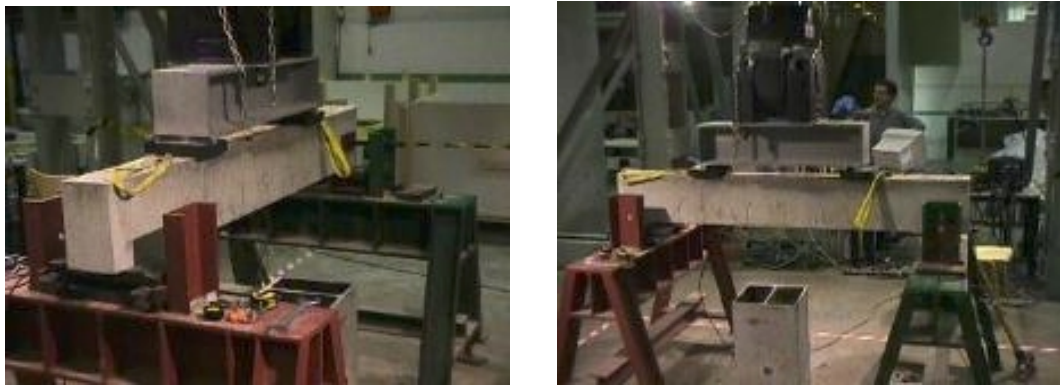
Figure 6.4.2. Pre-cracking before chemical attack.
