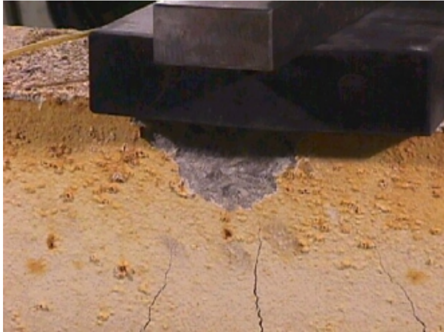
Figure 6.4.8. Neoprene interface between actuator and beam.
