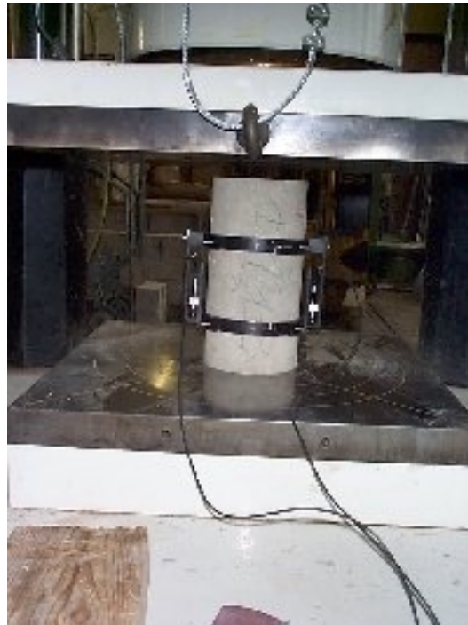
Figure 6.3.10. Strain controlled compressive test on cylinders to obtain static strain modulus.
