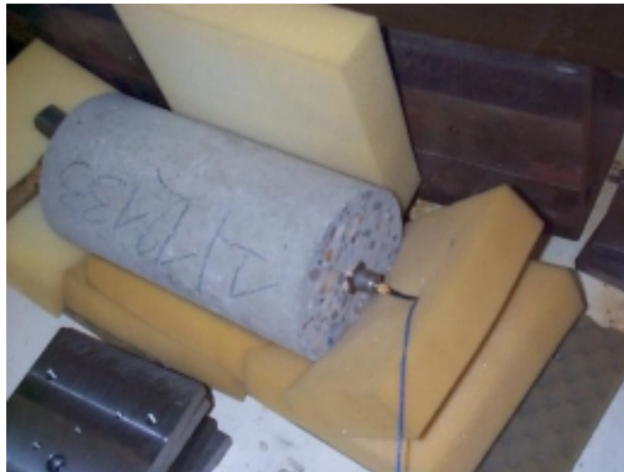
Figure 6.3.13 ASTM C-215 test to obtain dynamic strain modulus.
