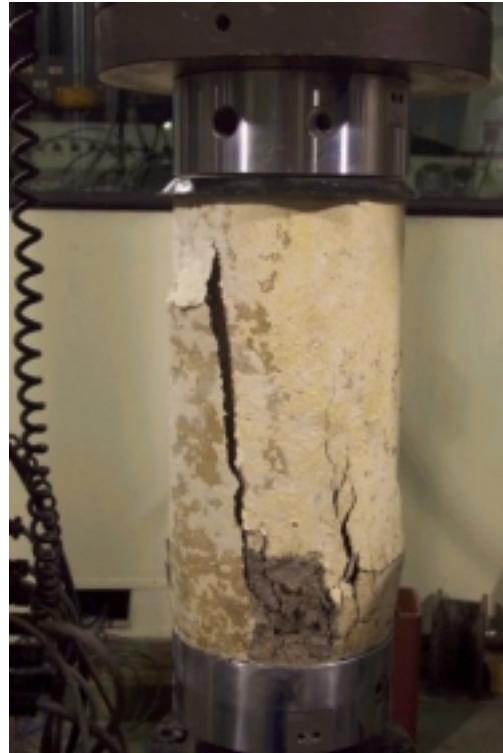
Figure 6.4.12. Compressive test on a 6-month SO 4 attacked cylinder.
