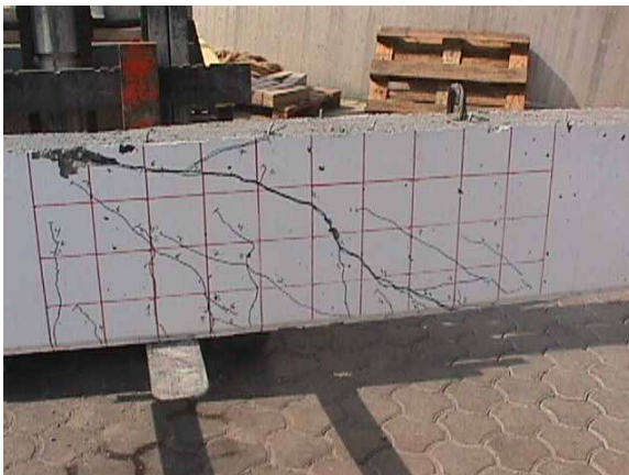
Cracking at failure ( V = 255.23 \text{ KN} )
