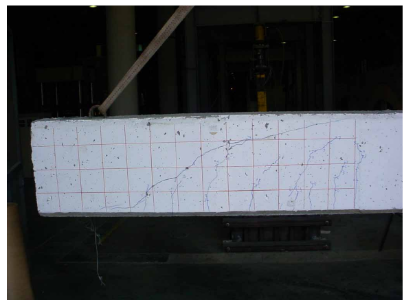
Cracking at failure ( V = 140.90 KN)
