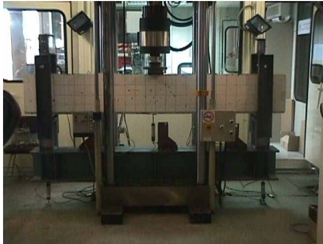
Test set-up for beam H75/1
