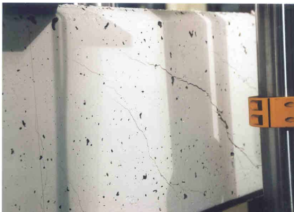
Shear crack prior to the beam failure
