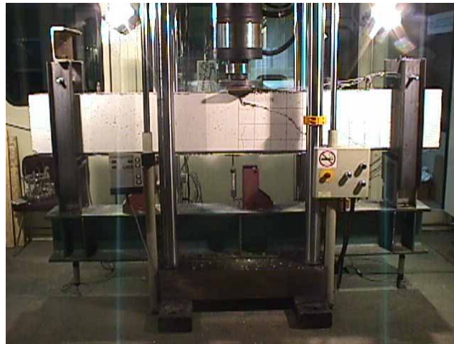
Test set-up for beam H60/4
