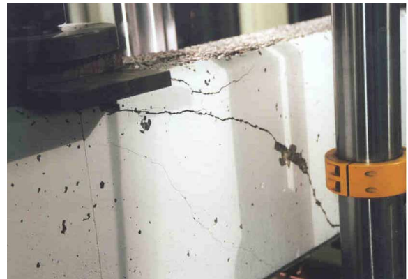
Detail of the shear crack
