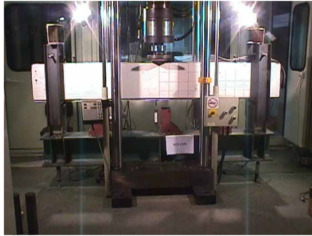
Test set-up for beam H75/2
