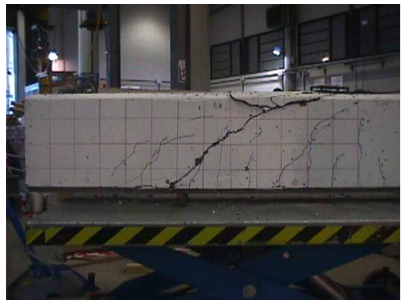
Cracking at failure ( V = 242.07 KN)
