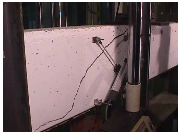
Cracking at failure ( V = 99.69 \text{ KN} )
