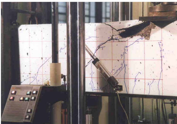
Cracking at failure ( V = 253.64 KN)
