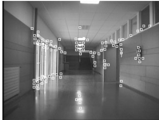
Figure A.4: Shi and Tomasi features over a typical mobile robotics scene.
