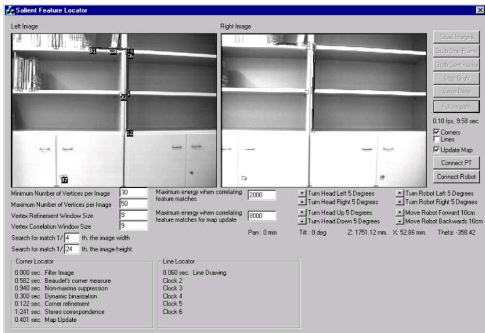
Figure 8.3: Graphical user interface for the extraction of visual landmarks from stereoscopic images.
