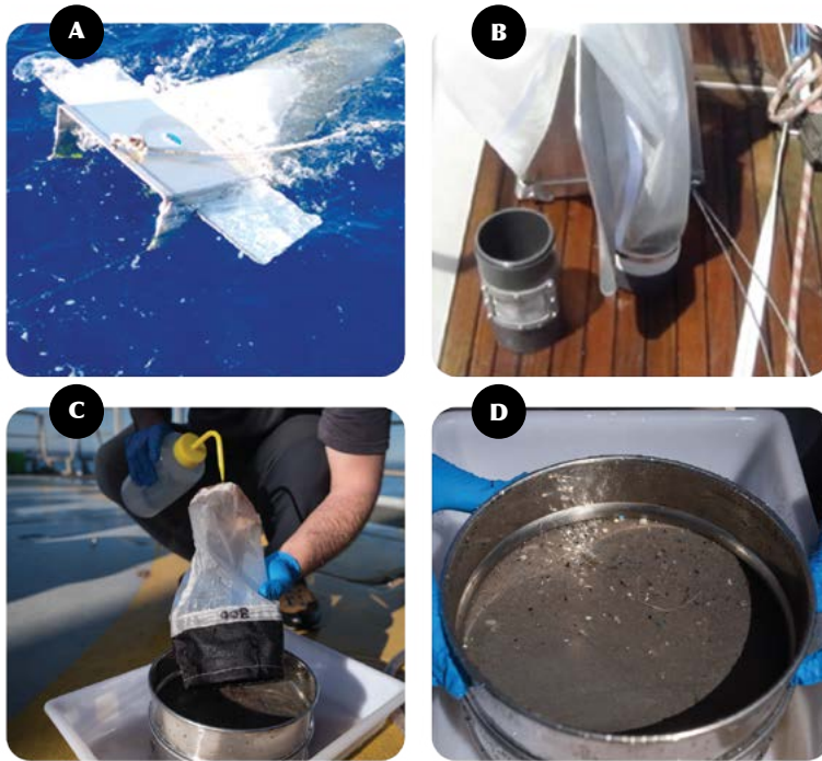
Figure 2.2. Example of the tools used during sampling. (A) Manta trawl net, (B) Net and cod-end, (C) transfer to the sieve, and (D) sample extracted in the sieve. (Image attributions: Chapter 10 - References).
