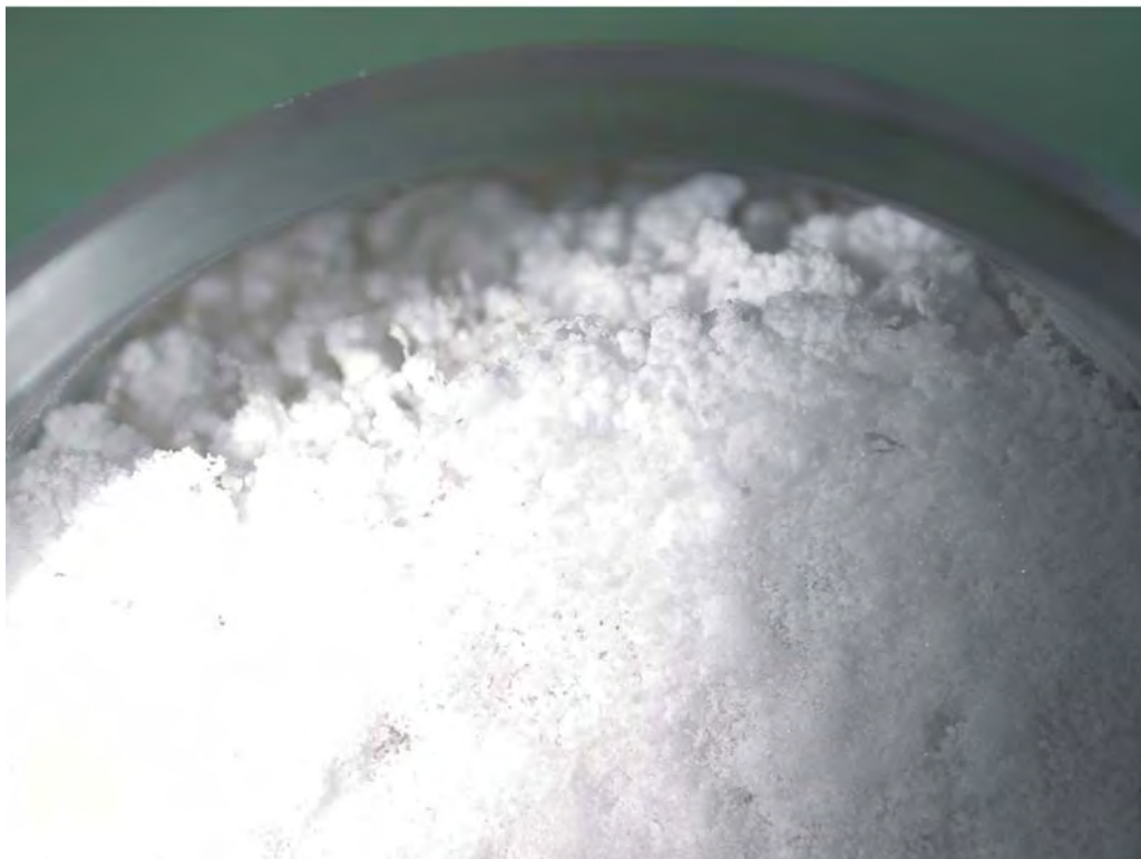
Fig. 4.16 Details of the cold end in the top of a sample after 30 days of application of the temperature difference.
