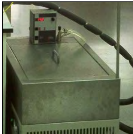
Fig. 4.9 Equipment from the HETO model “DT 1 CB 8-30 e” to keep the temperature constant in the cold side.
