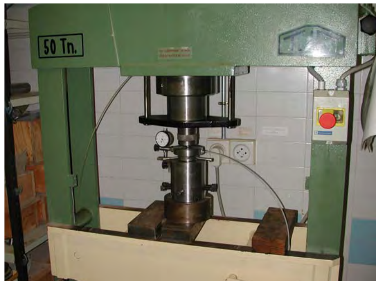
Fig. 3.10 Compactor during the preparation process.
