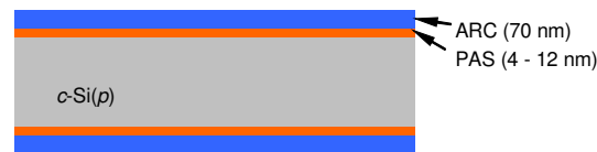
Figure 4.2. Schematic of the passivation structures by stacks of silicon carbide. PAS layer is Si rich with good passivation properties. ARC layer is C rich with good antireflective properties.
