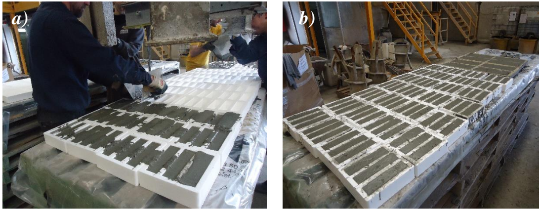
Figure 3.8 – Casting process: a) filling the moulds and b) final aspect of moulds after removing excess.
