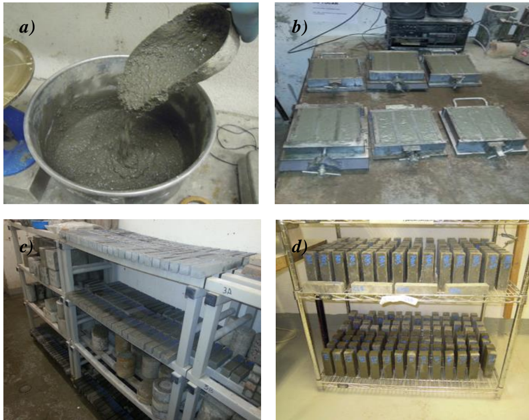
Figure 3.2 – Specimens preparation: a) mix prepared, b) mixes placed into metallic moulds, c) curing in the wet room and d) curing in the climatic room.
