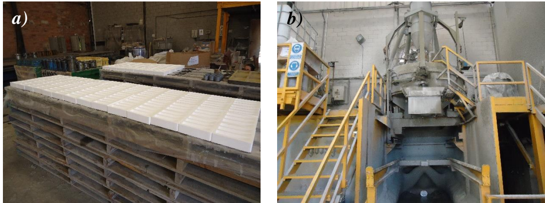
Figure 3.6 – Preparation of the specimens: a) moulds and b) vertical axis mixer.
