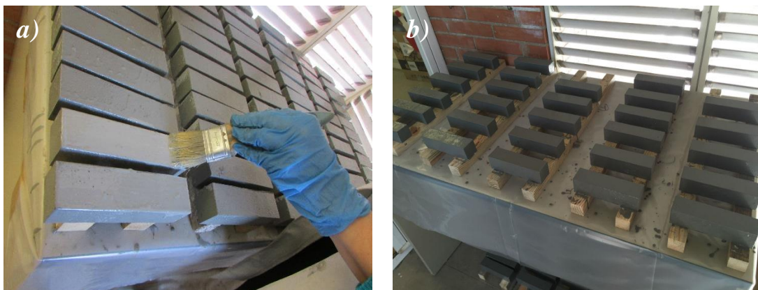
Figure 3.15 – Waterproofing the specimens: a) applying the epoxy membrane and b) curing of samples.
