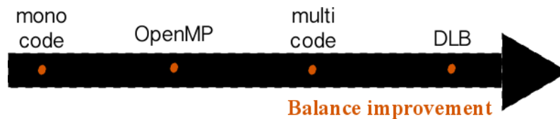
Figure 7.7: The balance of the code has improved in time including new parallelization and balancing tools.
