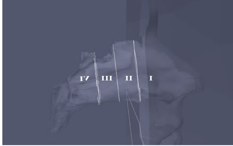
Figure 8.1: Splitting the nose domain in different zones for an easier study of particles deposition.
