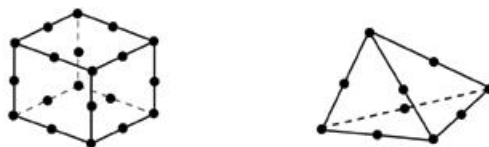
Figure 3.7: Two examples of quadratic elements: on the left, a 20-node brick, on the right a 10-node tetrahedron.
