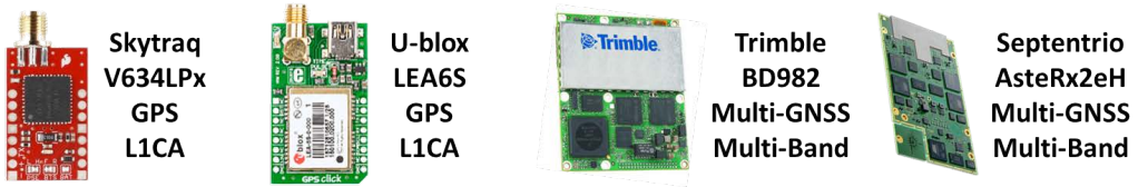
Figure 10.8: GNSS receivers used in the real-time RFI mitigation performance tests of FENIX-Lite.
