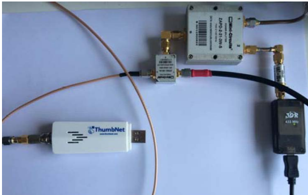
Figure 11.9: Setup used to evaluate the robustness of the FHSS modulation with real signals.
