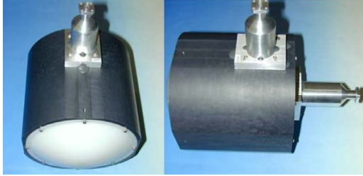
Figure 4.3: Corrugated horn with its Fresnel lens used in the Ka-band with the corresponding output waveguides for V and H polarizations.
