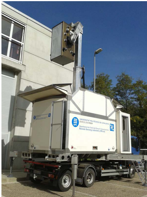
Figure 4.7: MERITXELL assembled to the telescopic robotic arm above the housing structure and the truck.
