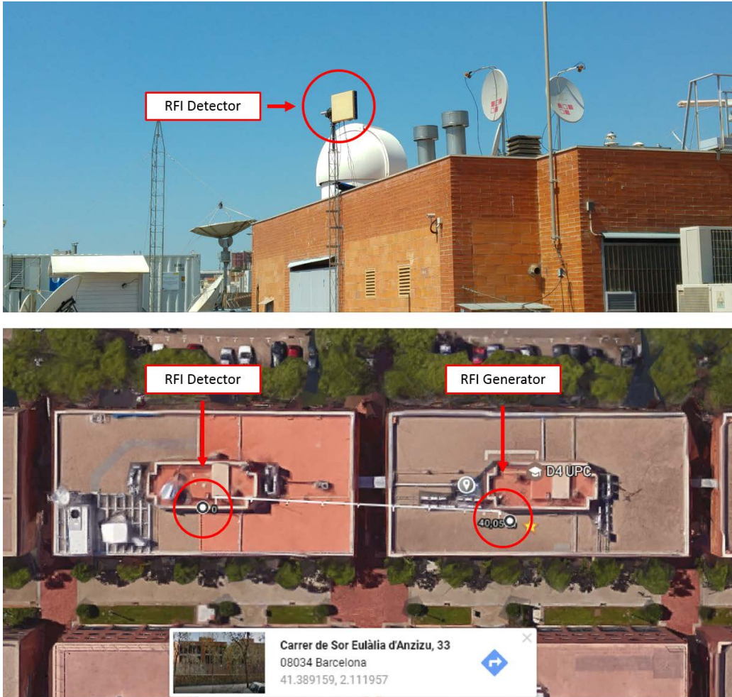
Figure 6.8: RFI detector attached to the mast (top). Experiment location with 40 meters between RFI detector and generator.
