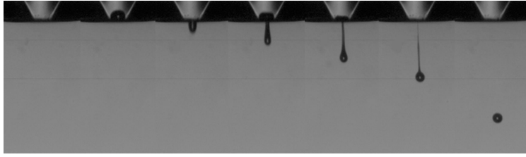
Figure 3.2: Sequence of images of a drop generated by a piezoelectric actuator.
