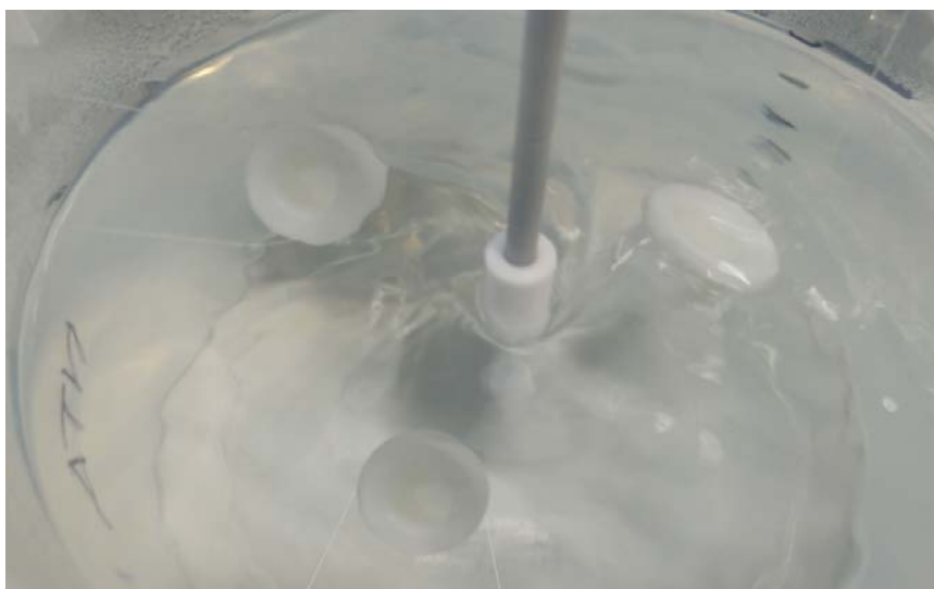
Figure 6.3. Picture of a typical experimental setup, showing three samplers suspended from plastic wires, left free to float in a stirred solution.
