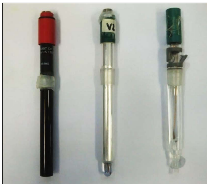
Figure 2.1. Electrodes used for the potentiometric measurements: Cd-ISE Crison 9658S7, Separate pH electrode Metrohm 6.0133.100 and Ag/AgCl reference electrode Metrohm 6.0726.100.
