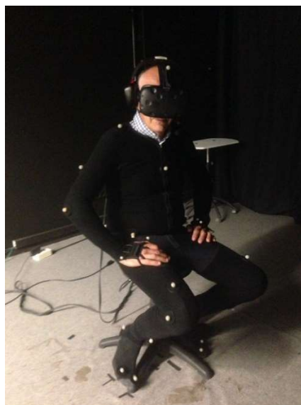
Figure 4: A participant wearing the Optitrack body suit and the HTV VIVE Head Mounted display
