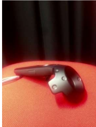
Figure 3: Hand controller of the HTC VIVE, in experiment II and III participants were holding one controller in each hand in order to track their upper body movements and map them to their virtual body in real time
