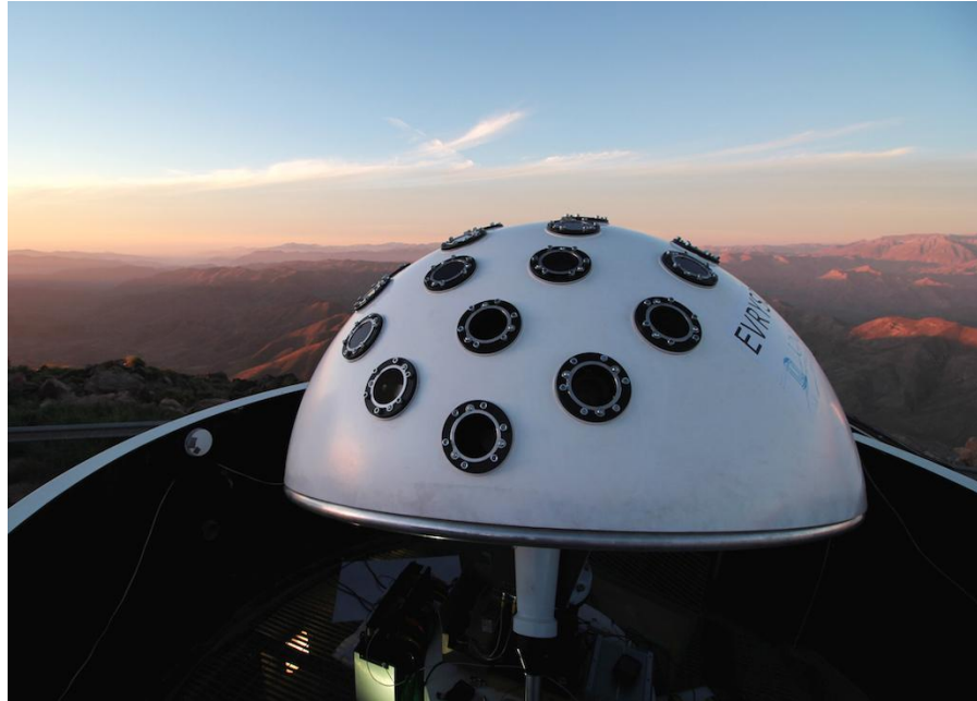
Figure 26: The Evryscope deployed at CTIO . The main dome is 6 feet in diameter. The system is mounted inside an AstroHaven dome maintained as part of the PROMPT telescope network.
