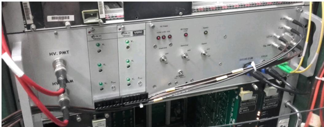
Figure 5.44 – Back-End prototype integration into a 6U EuroCard subrack chassis.
