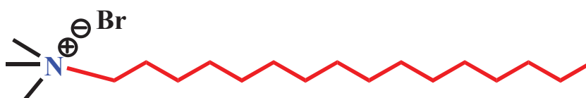
Scheme 2.1. Chemical structure of cetyltrimethylammonium bromide.
