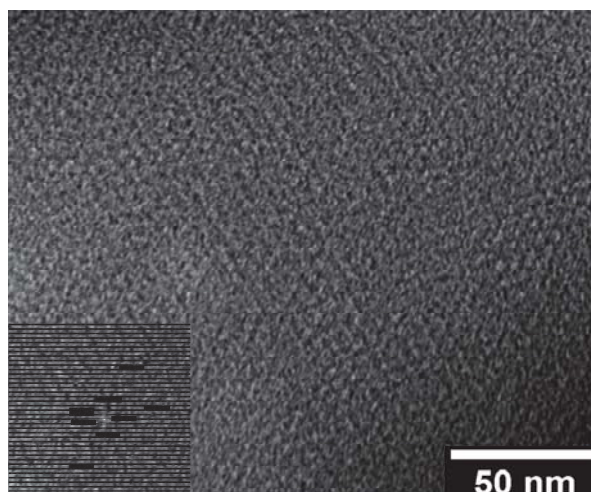
Figure SI-5. TEM micrograph from a film of 18ACh·HyA complex. Inset; OD pattern indicating the periodical spacing displayed on the film.
