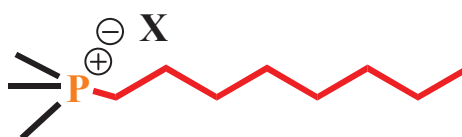
Scheme 2.3. Chemical formula of tetraalkylphosphonium salts containing one long alkyl chain.
