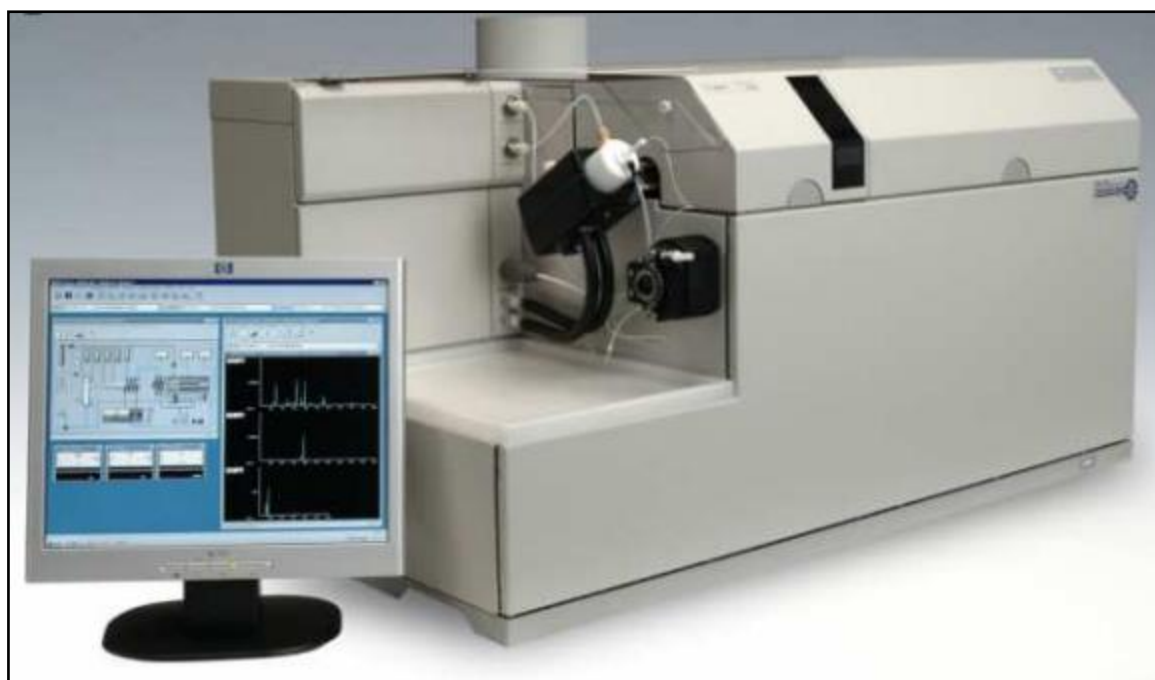
Figure II.14: ICP-MS de type Agilent 7500c
