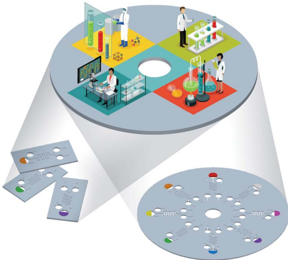
Figure 1.2: The “Lab on a Chip” concept. Several “lab” functionalities can be implemented in a single microfluidic platform.
